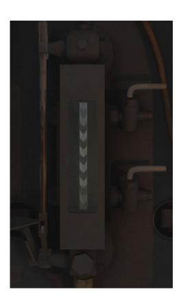
Attached to the boiler is a strong glass tube indicating the current level of water in the boiler. If this reaches the bottom then the fusible plugs will melt and relieve the boiler pressure whilst providing a warning to the locomotive crew.
