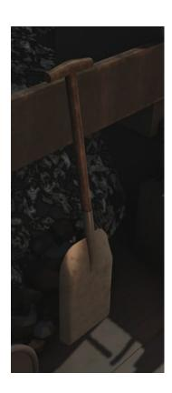
The shovel on the tender is used to control the stoking speed/amount.
